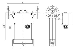
**Process Connection** Face to face length (L) Order Code in mm ANSI ½" 150# RF 220 8.66 A1 ANSI 1/2" 300# RF 220 8.66 A2 ANSI ½" 600# RF 220 8.66 Α3 ANSI ½" 1500# RF 300 11.81 A6 ANSI ½" 1500# RTJ 300 11.81 R1 DIN DN15/PN40 220 8.66 D1 DIN DN15/PN100 220 8.66 D2 DIN DN15/PN 160 220 8.66 20 JIS RF 10k 15A (½") 220 8.66 J1 JIS RF 20k 15A (½") 220 8.66 J2
