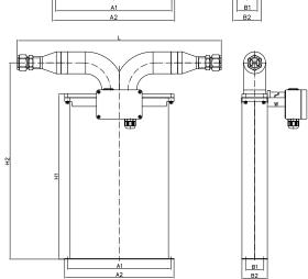
The sensor is manufactured with two internal measurement tubes arranged side by side. In parallel or dual path sensors, these tubes are connected in parallel and the flowing fluid is split equally between them. For customization of face to face length and/or special fittings other than the ones listed on this page, please consult factory.
